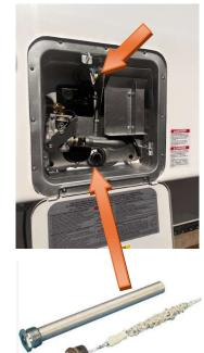
7. In the termination compartment you will find the Water pump/fresh water supply shut off valve and the Antifreeze pickup port and shut off valve.
