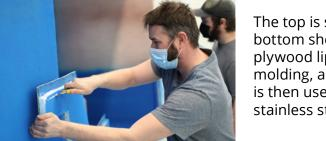
The top is screwed onto the bottom shell through this plywood lip. Using a metal molding, a vinyl insert is then used to cover up stainless steel screws.
