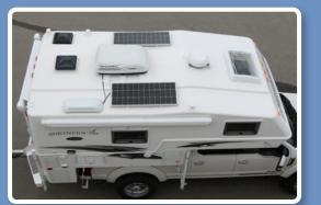
Dual 100 Watt Solar Panels on LE and SE
