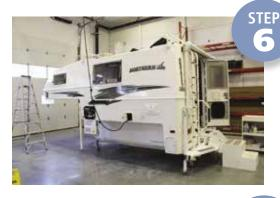
At the Final Inspection station, final finishing is completed and quality and systems checks are carried out.
