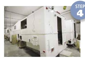
The camper then proceeds to the assembly line where openings for doors, windows, and exterior compartments are cut out and assembly begins.
