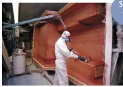
After a layer of Gelcoat is applied to the interior of the mold, a mixture of "chopped" fiberglass strands and a plastic resin is sprayed on top of the Gelcoat to form a very rigid, strong and light weight molded shell.
