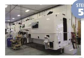
As the camper moves down the assembly line, cupboards, cabinets and appliances are installed and the exterior is completed.
