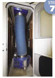
Air pressure testing is the final test before the camper leaves the assembly line.
