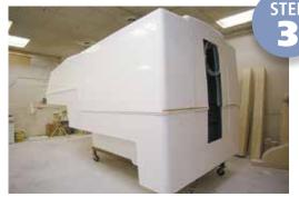
The top is screwed onto the bottom shell through this plywood lip. Using a metal molding, a vinyl insert is then used to cover up stainless steel screws.
